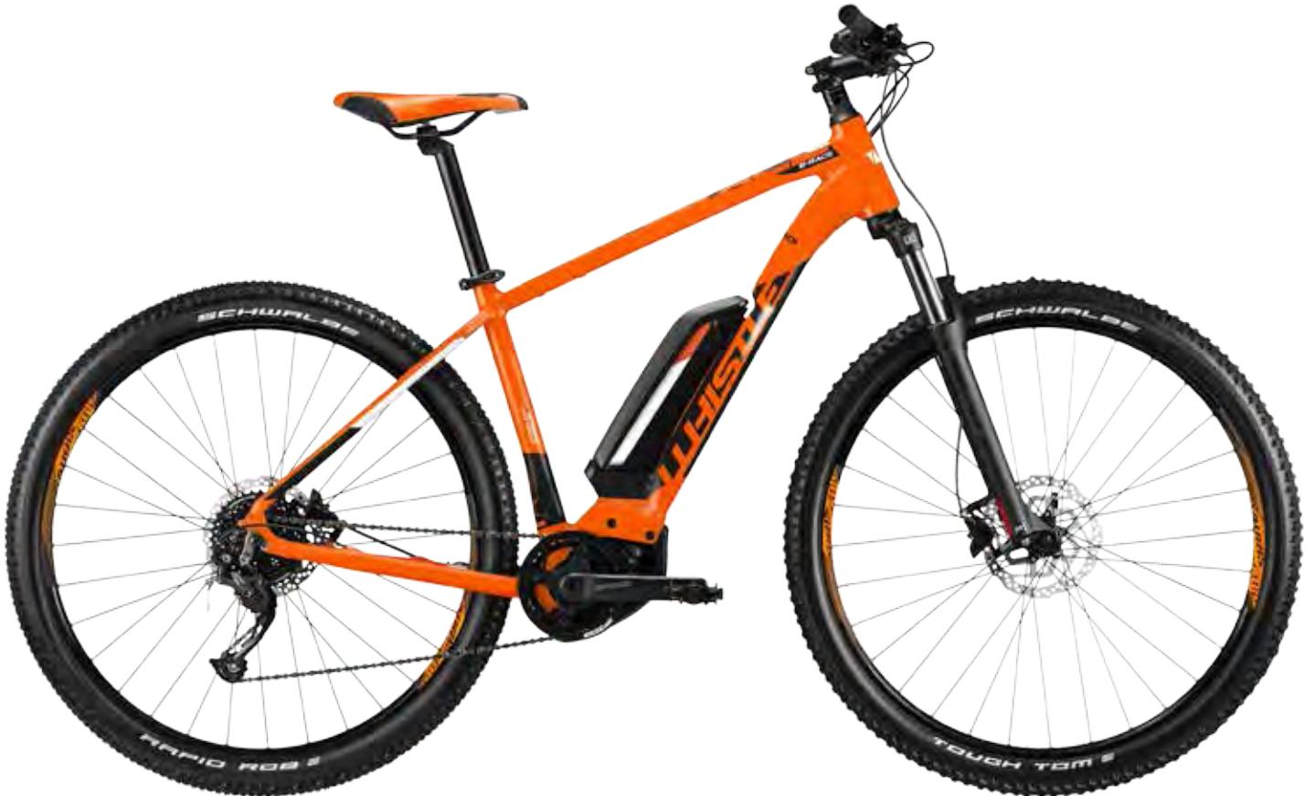
FRAME Alu 29", hydroformed, custom tubing, Internal Routing, Forged interface
