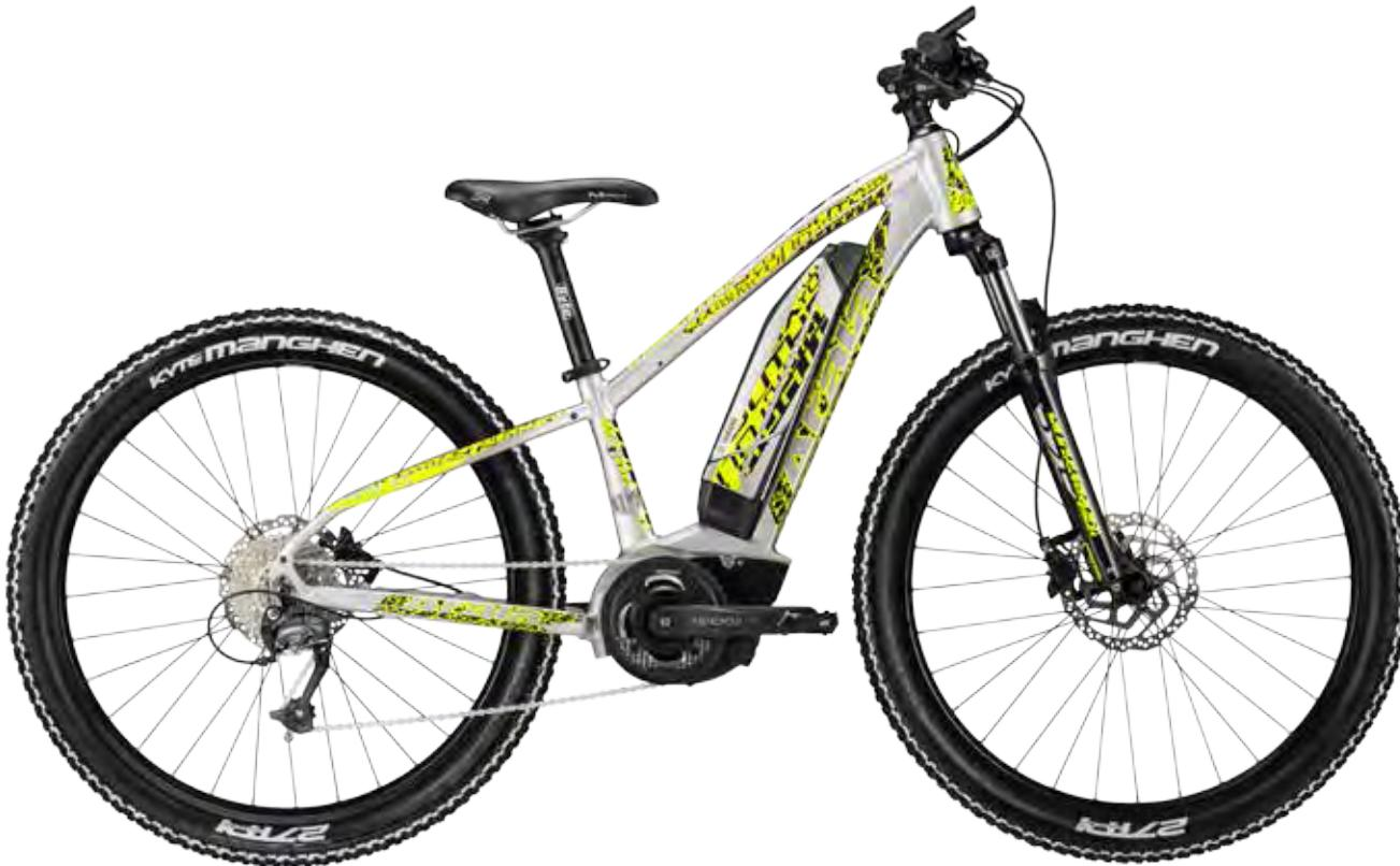
**FRAME** Alu 27,5", custom tubing, tapered, Internal routing, Forged interface
