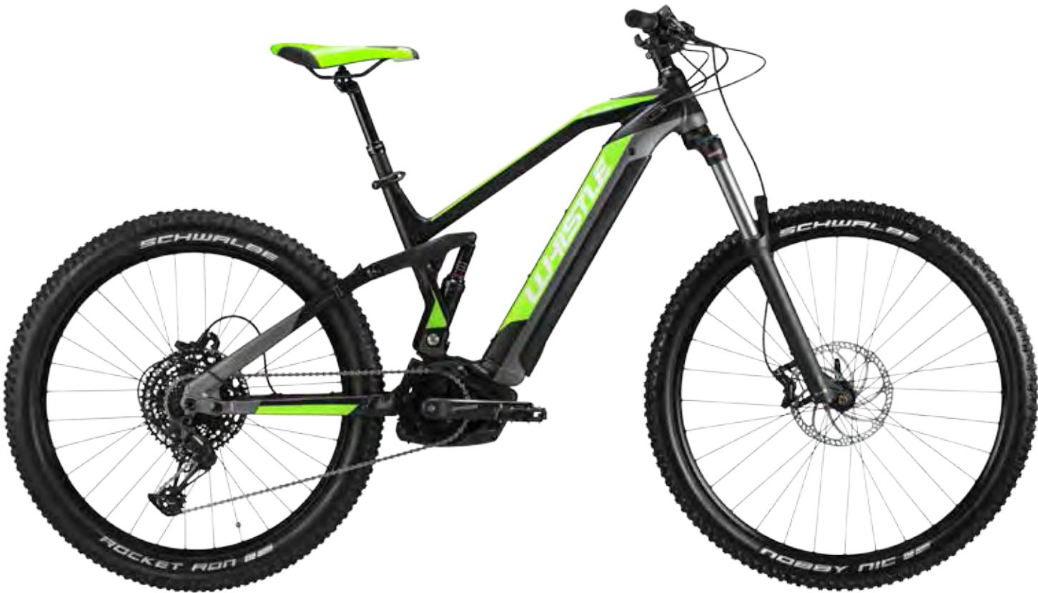
**FRAME** Alu, 27,5"+, hydroformed, integrated battery, tapered, Rear travel 150 mm, 12x148 mm, Gravity casting interface
